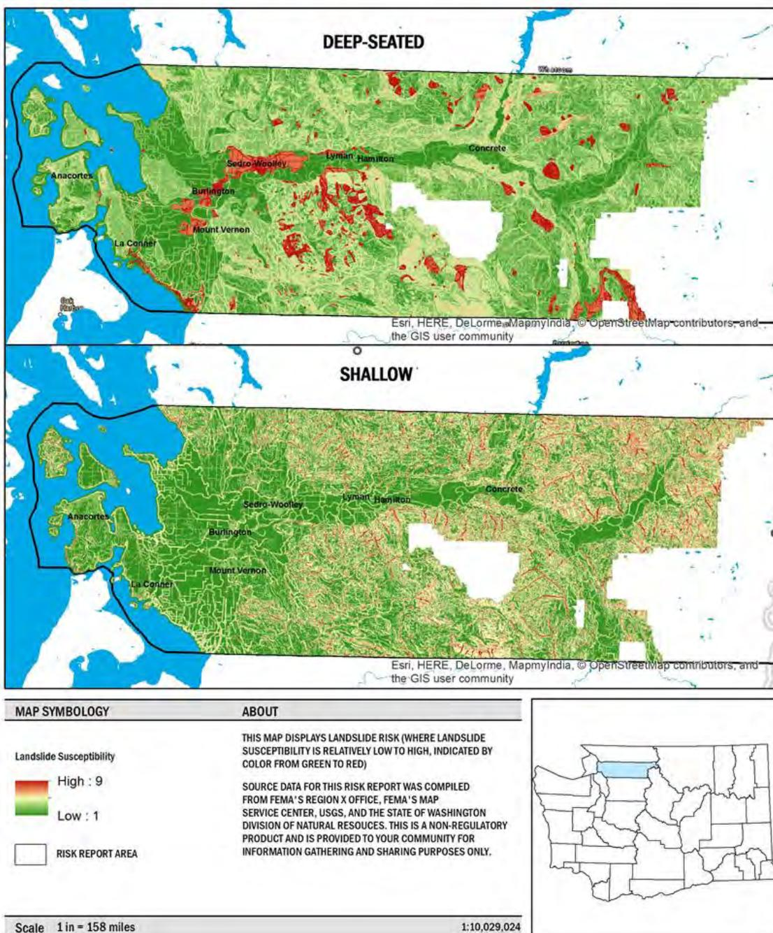
Figure 8-14 Landslide Susceptibility Zones (FEMA, 2017)
