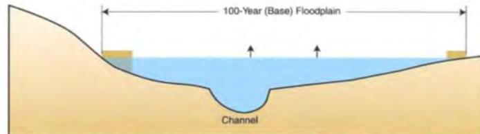
The computer model simulates what happens when the edge of the floodplain is filled or otherwise obstructed. The base flood elevation will increase because there is less room for floodwaters.
