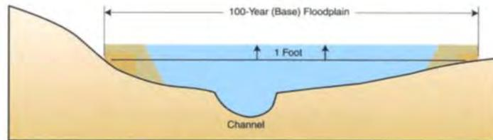
The simulated obstructions are moved closer to the channel. The model notes when the flood elevation increases by 1 foot.
