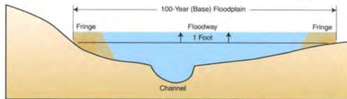
The point where obstructions on the edge of the floodplain cause a 1 foot increase determines the location of the floodway boundary. The area where fill is allowed is called the floodway fringe.
